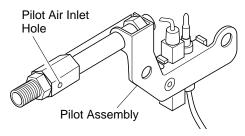
Figure 22 - Pilot Inlet Air Hole
